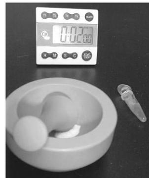
**Figure 2: Mortar and pestle with sample, timer, and plastic vial.**
