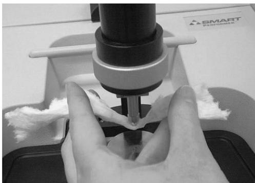
**Figure 17: Removing sample from the tip of the pressure applicator.**
